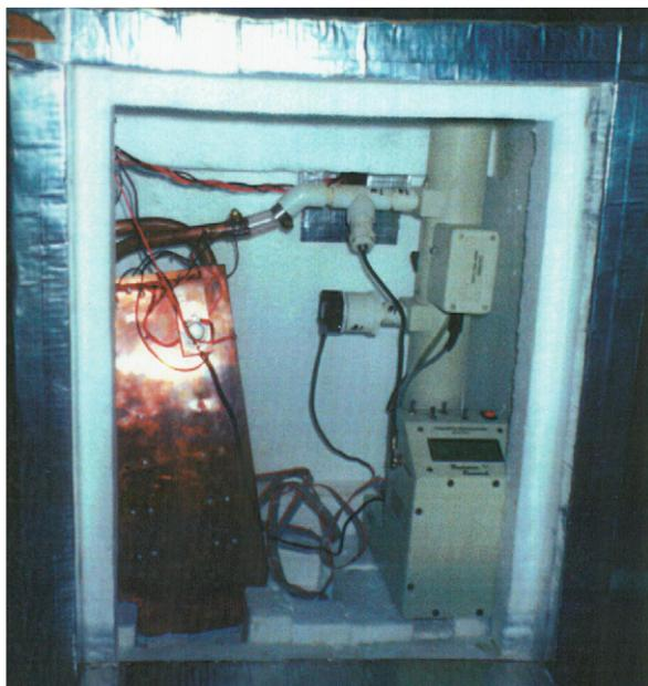
Photo 1. Insulated box with front cover removed, showing air intake through heater (left) to the RR neph (right).
