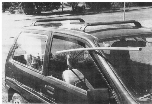
Photo 2. Inlet pipe to the nephelometer positioned through the top of the front driverside window, facing forwards, so the vehicle's motion aided the fan in drawing air through the instrument.
